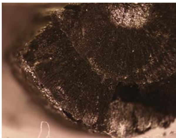
Fig. 12. Cross-section of common alder ( Alnus glutinosa ) from Sample 1 (ID 1.2). The size of the sample is 9 × 10 × 9 mm (©Máté Róbert Merkl)
