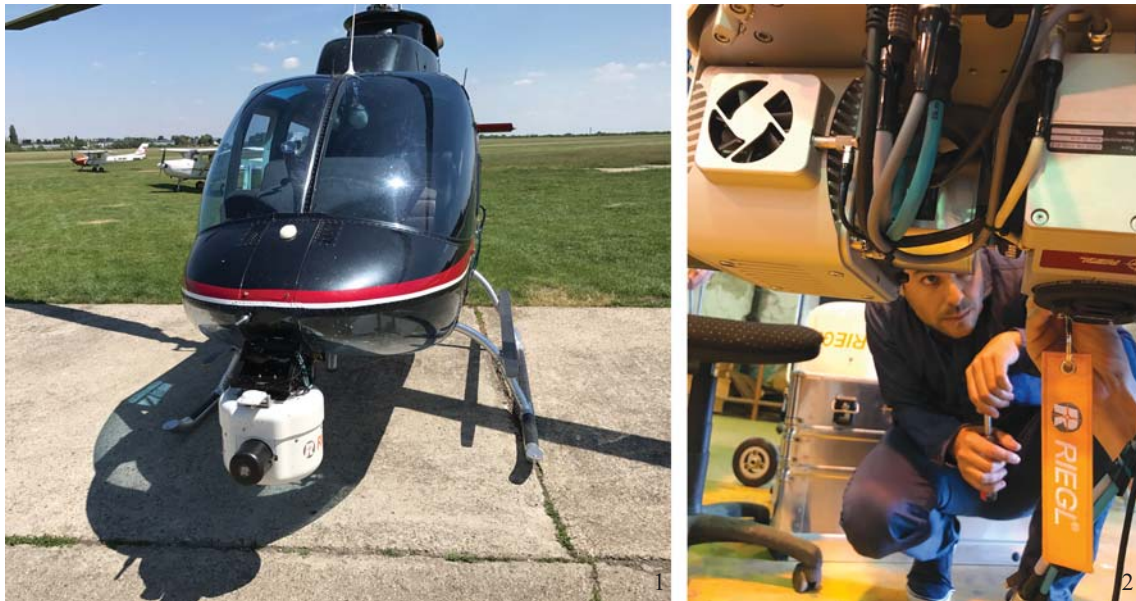
Fig. 1. 1. Riegl VP-1 VUX LiDAR laser scanner; 2. Riegl VP-1 VUX LiDAR laser scanner mounted on a helicopter
